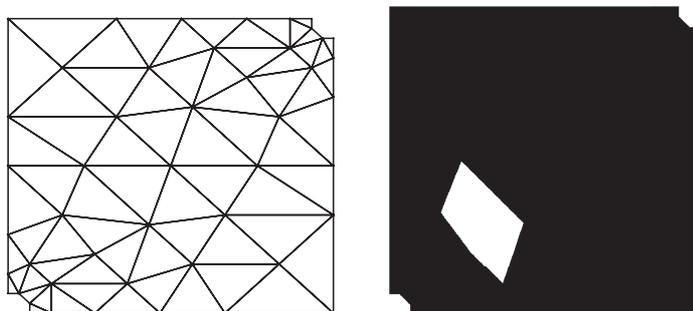
FIGURE 1. Unstructured triangular mesh (left) and permeability field (right):  $k = 10^{-12}m^2$  in white regions and  $k = 10^{-8}m^2$  in rest of domain.
