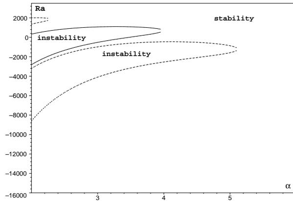
FIGURE 1. Marginal curves of  $Ra$  versus  $\alpha$  for synchronous (solid line) and subharmonic (dashed line) modes, obtained by the method of continued fractions;  $\omega = 30$ ,  $\eta = 3$ ,  $R_s = 3000$ ,  $Le = 1$ .
