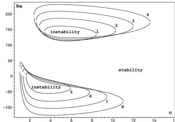
FIGURE 2. Marginal curves of  $Ra$  versus  $\alpha$  for large  $\omega$ , obtained by the method of averaging for the case of monotonic instability;  $\eta/\omega = 0.3$ ,  $Le = 3$ . Curves 1–8 correspond to 1)  $R_s = 163$ , 2)  $R_s = 183$ , 3)  $R_s = 203$ , 4)  $R_s = 223$ , 5)  $R_s = -59$ , 6)  $R_s = -79$ , 7)  $R_s = -99$ , 8)  $R_s = -119$ .
